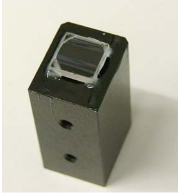
Lens glued in the correct orientation onto the block.
