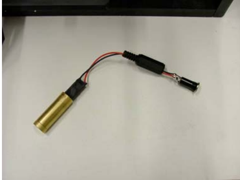
Female 3.5" Jack socket soldered.
