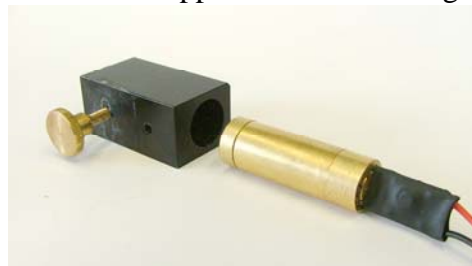
Bottom of the mounting block with adjust screw.
