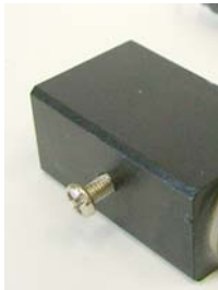
Top of the mounting block with laser securing screw.
