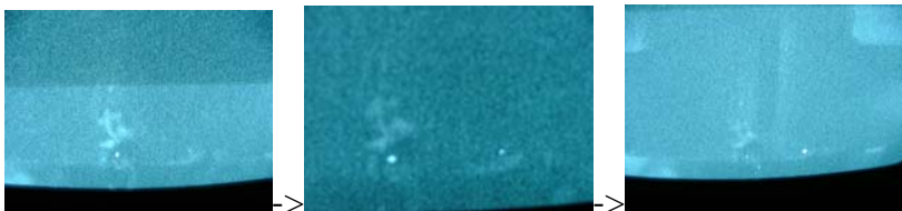
Roll the Drop Delay Knob to see all the beads deflected to the right
