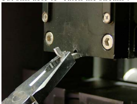
Bending the Centre Catch Tube with pliers.
